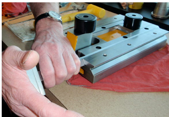
FIGURE 11: Checking for proper loading on the bearing cage using a dull putty knife
