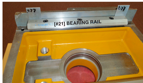
FIGURE 7: Bearing Rail tight against parallel blocks for loading internal gage bearings
