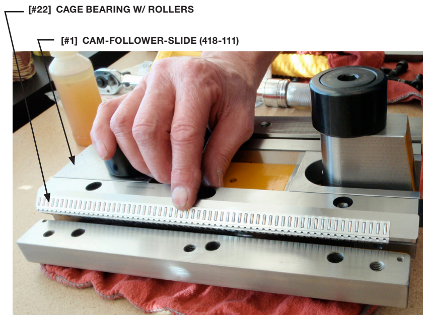
FIGURE 5: Installing cage bearings with rollers for the internal slide
