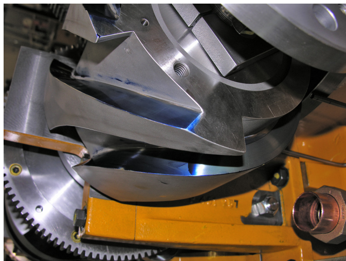
FIGURE 13 — GOOD PATTERN OF TRANSFER TURRET CAM ON ALL SURFACES
