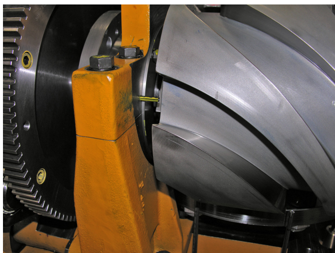
FIGURE 1 — CAM POSITION FOR ALIGNMENT PROCEDURE
